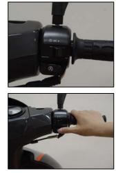
Press down starter switch button to use electric starter.
