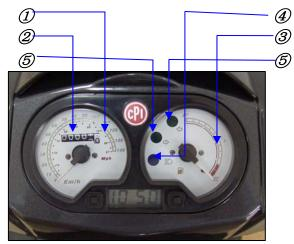
1.Speedometer:Forward speed is based on 1km per hour.
