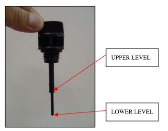
**B.GASOLINE:** 1.Gasoline inspection / replenishment:
